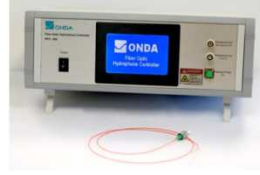
Type: Fiber optic hydrophone
